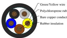
Polychloroprene rubber outer jacket Bare copper conductor
